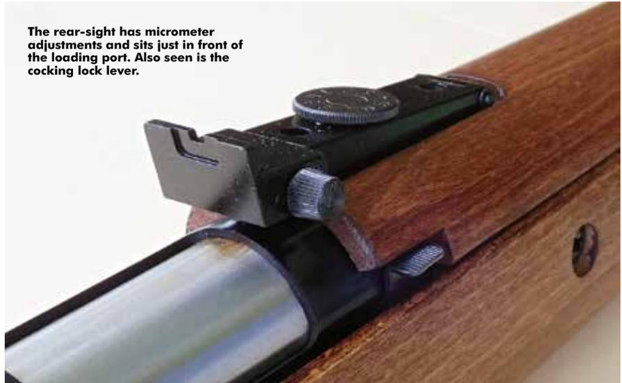
The rear-sight has micrometer adjustments and sits just in front of the loading port. Also seen is the cocking lock lever.
